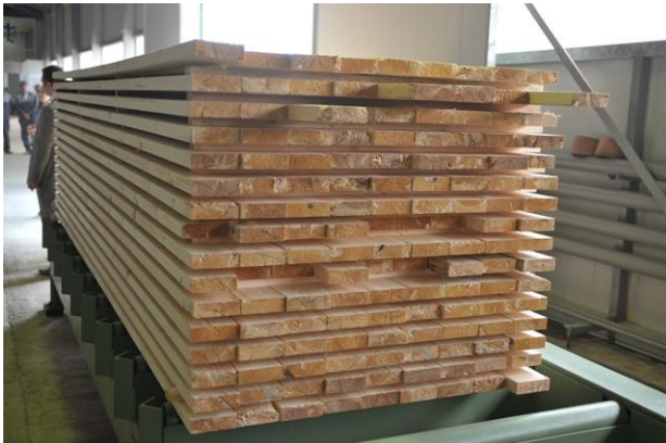
Boards stacked automatically on sticks to get packages ready for drying
